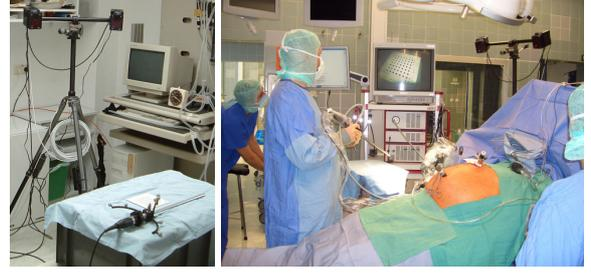
Figure 6: Left: Optical tracking system smARTtrack1 in the laboratory. Right: smARTtrack1 in the operating room during an endoscopic surgery. Images by courtesy of F. Vogt.
